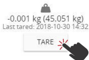
By default, the graph of the **Weight Sensor** will display measurements of a tared weight. To display the untarred
